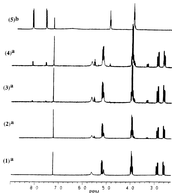
Figure 1. ^1\text{H-NMR} spectra were recorded with a Bruker AM 360 MHz in \text{CDCl}_3 (0.6 mL) with one drop of \text{AcOH-d}_4 . (a) (1), (2), (3), and (4) were spectra of 1b recorded at intervals of 0, 1, 3, 7 days; (b) (5) is the spectrum of 3b .
